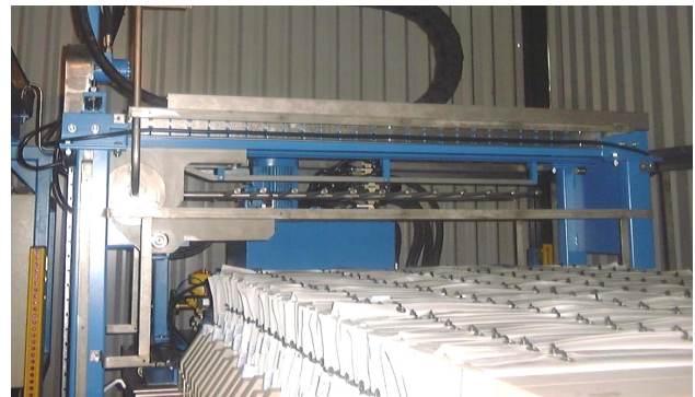
Cloth Washing Machine Fitted to a 1500mm Sq Sidebar Filter Press
