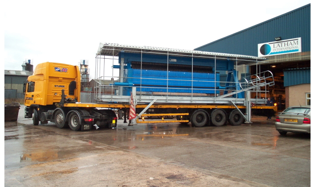
Mobile Filter Press, Jack on, Jack Off Future Industrial Services, UK
